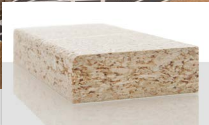
1. Highly porous middle layer of chipboard prevents wrapping with thin paper foils.
